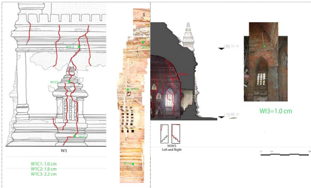
Fig. 8 (left), Fig. 9 (right) The digital documentation of two corresponding cracks on the exterior and interior wall of a monument.
