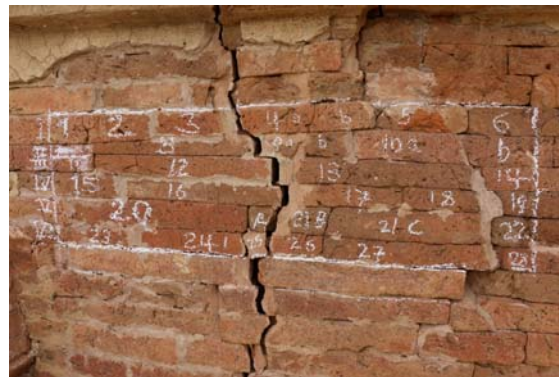
Fig. 20 Test panel of a Bagan monument with individually numbered bricks. For each brick the rebound-hammer test is applied at least three times and noted down in the field notes. The ultra-sonic test is also undertaken in order to determine the overall compactness of the entire brick masonry panel. (Source: ©UNESCO/AMA/DoA)
