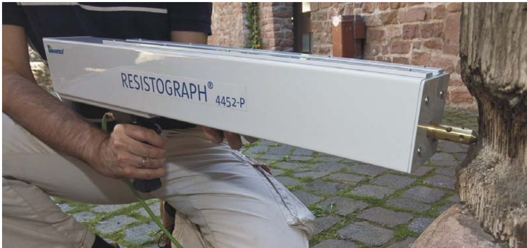
Fig. 19 The use of resistograph on timber during the building investigation.
