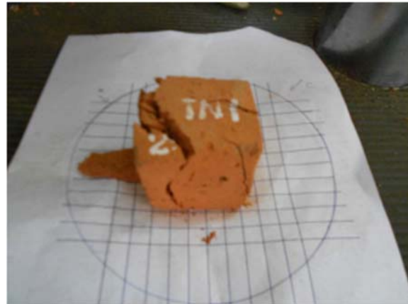
Fig. 62 (right) Compression test of a brick sample, provenance “TN”, situation after the collapse.
