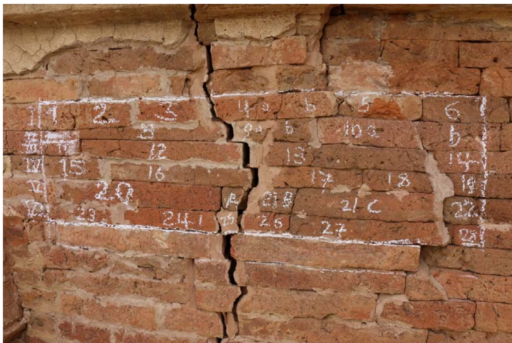
Fig. 48 Test panel no. 4 for which the rebound hammer test was applied three times for each individual brick to test their compression strength, as well as, the ultra-sonic test to determine the compactness of the overall masonry panel.
