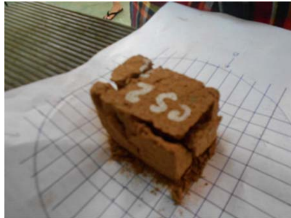
Fig. 66 (right) Compression test of a brick sample, provenance “ES”, situation after the collapse.
