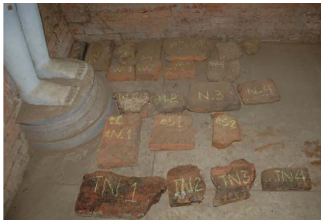
Fig. 15 Bricks are neatly arranged and their suitability for laboratory testing is tested by applying the rebound hammer before packing them carefully to be taken to the laboratory in Yangon. Any kind of vibration that could impact the strength of the bricks should be avoided during transport.
