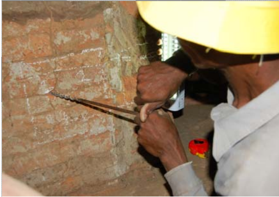
Fig. 22 A hand drill is used to make a whole into the wall of a monument through which the condition and composition of the wall can be investigated with an endoscope.
