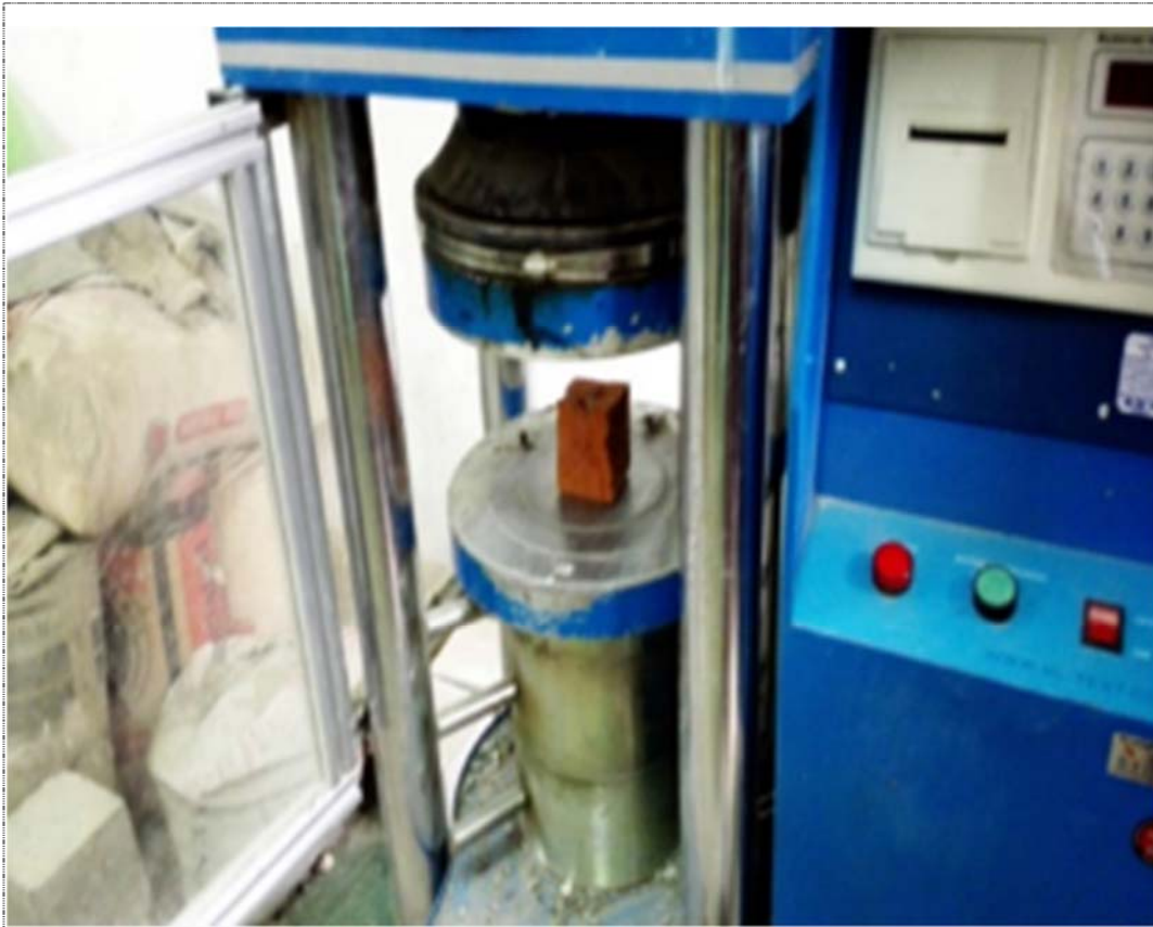
Fig. 55 Sample of brick under the machine before the test.
