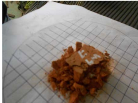
Fig. 64 (right) Compression test of a brick sample, provenance “W”, situation after the collapse.
