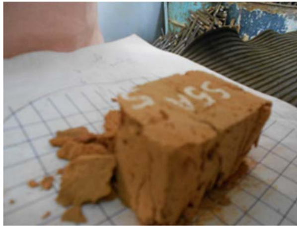
Fig. 56 (right) Compression test of a brick sample, provenance "S", situation after the collapse
