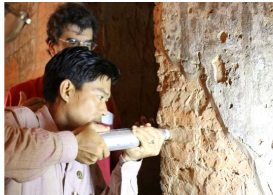
Fig. 18 A DoA staff member using a rebound hammer. The plunger should be pushed in a 90-degree angle against the testing surface. When the plunger makes the impact on the surface the locking button has to be pressed. Afterwards, the rebound value can be read from the scale.
